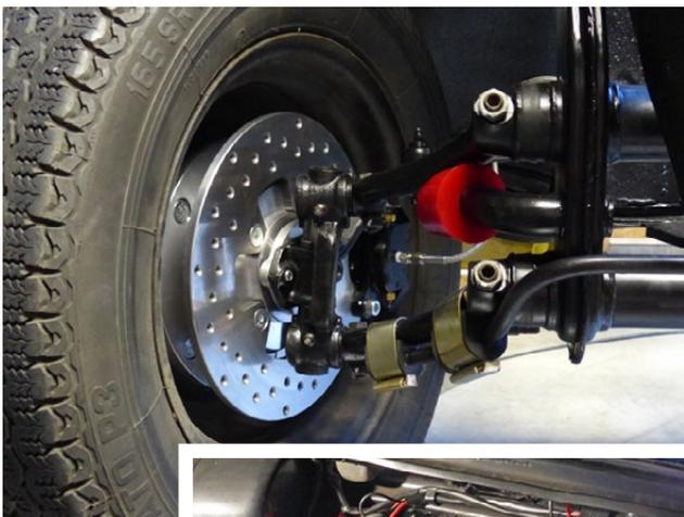
Front disc brake and axle beam
