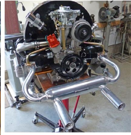
The engine displacement has been raised from 1200cc to 1776cc. A fully rebuilt and strengthened transaxle, sourced from Southern California has been installed. Disc brakes have been fitted at the front, activated by a dual master cylinder. Heavy duty torsion bars and shock absorbers and a raised, adjustable front axle beam have been fitted. Additional reinforcements have been added to the suspension components.
