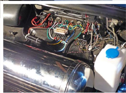
Additional wiring, fuel tank and even a windshield washer system
